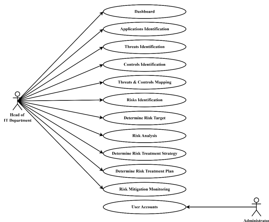
Figure 5. Use Case Diagram for the Risk Mitigation Prototype.
